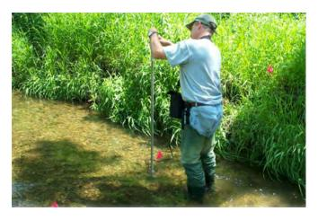
Fig. 6. Measuring flow velocity at a stream restoration monitoring site.
